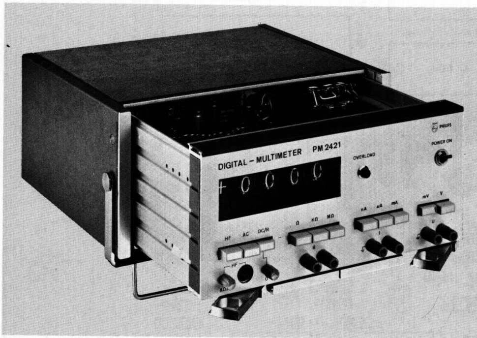
Fig. 42. Pulling the instrument chassis out of the cabinet
